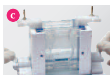
Transfer to casting base and tighten cams.
