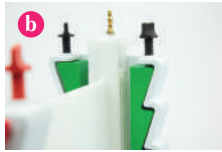
Loosen the vertical screw-pins in the PAGE insert to release the locking mechanism. This allows the gel clamps to sit in the resting slots.
