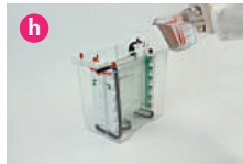
Transfer the PAGE insert to the gel tank. Fill the inner and outer buffer chambers before loading samples.
