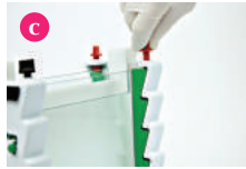
Insert a gel cassette into each side of the inner buffer chamber in the PAGE insert and tighten the vertical screw-pins.
