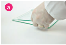
Assemble each gel cassette on flat surface, by placing the plain glass plate down with the spacers facing upwards followed by the notched glass plates.
