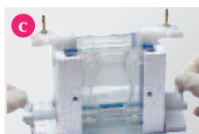
c Transfer to casting base and tighten cams.
