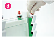
Continue to tighten the screw-pins until the gel clamps glide out of the resting slots and fix firmly against the glass plates pushing them upright.
