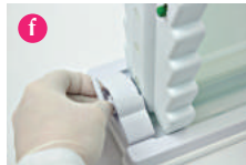
Insert cams and turn until tight, drawing the PAGE insert onto the casting to form a leak-proof seal.
