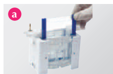
a Insert glass plates between pressure frame and gasket.
