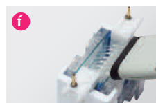
f Load samples using Loading Guides and run.
