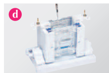
d Insert gel solution and comb. Allow to polymerise.
