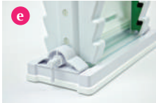
Check the bottom of the glass plates to ensure that they are even together and place the PAGE insert onto the casting base. Make sure the cams are facing downwards.
