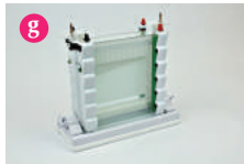
Pour in the gel solution, insert the combs and allow the wells to polymerise.
