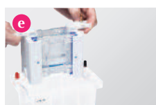
e Transfer to tank and fill with buffer.
